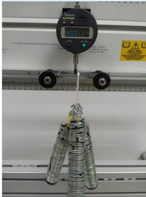
Figure 4 : The bending test machine with a loaded composite sample
